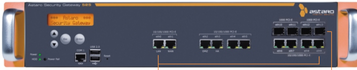
10 x 10/100/1000 Base-TX (copper) 4 x SFP GBIC (fiber or copper)
